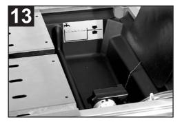
Before any cutting operation, make sure that the water level inside the basin is correct. (See picture 13)
