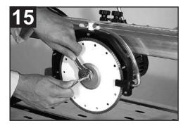
After dismantling the blade, clean the blade flanges carefully and check them for wear.
