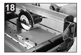
THE MILLIMETRE RULER PLACED ON THE WORKING TABLE HELPS ONLY WITH THE CARRYING OUT OF LINEAR CUTTING.
