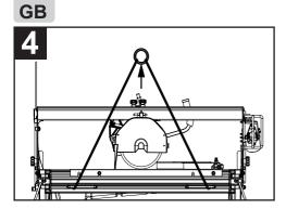
To move the machine, use a four-arm tie rod with the capacity to lift 200 kg or at least 20% more than the machine weight, by making use of the hooks in the transport handles (see picture 4).
